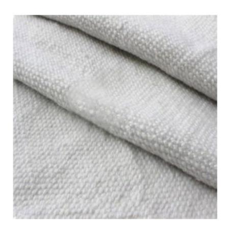
Ceramic Fiber is a narrow woven fabric manufactured from high temperature alumino-silicate based ceramic fiber reinforced with stainless steel wire. The product is white and odorless, suitable for high temperature applications up to 2300°F.
